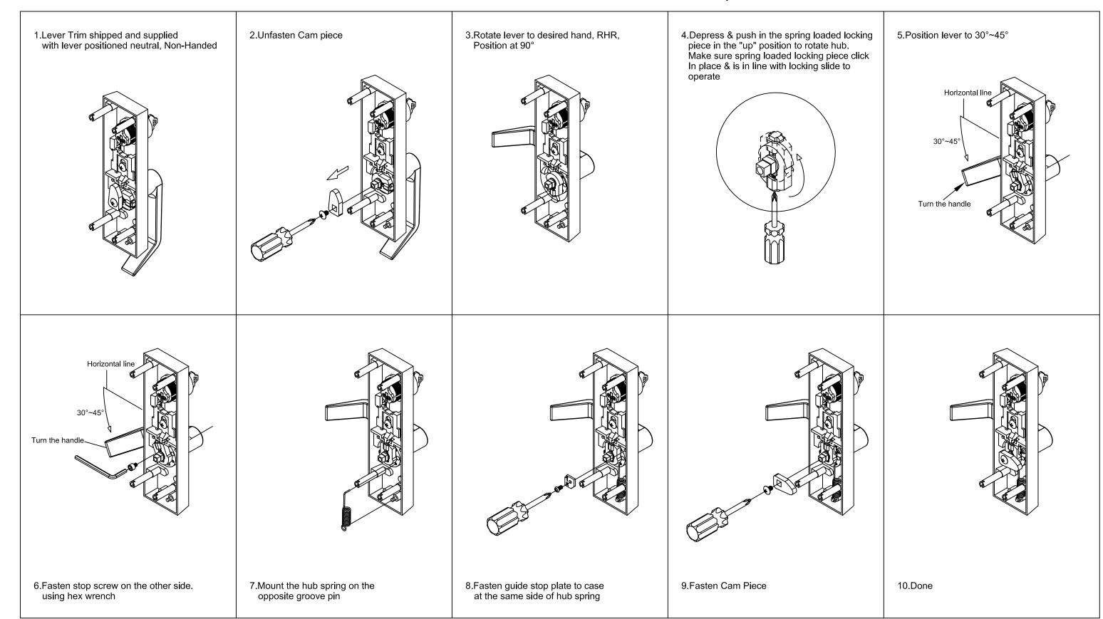
Method for replacing cyl
